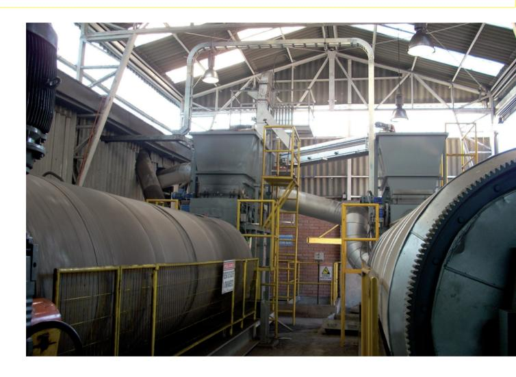
The GRINDING STATION is composed of one or more rotational grinders to dry and micronise the solid fuel and a storing silo.
