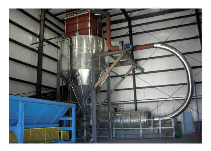
After drying and grinding, the fuel is sent to the silo though a bag filter to ensure a dry storage
