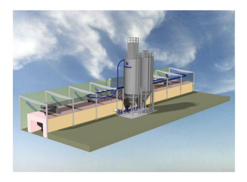
The MICROMATIC system works on the same basis as the PROMATIC system as far as fuel distribution and injection is concerned. The access to ready-micronised fuel allows to do without a grinding mill which is replaced by storage silus that feed the distribution circuit. To date, more than 20 installations have been successfuly put at work.
